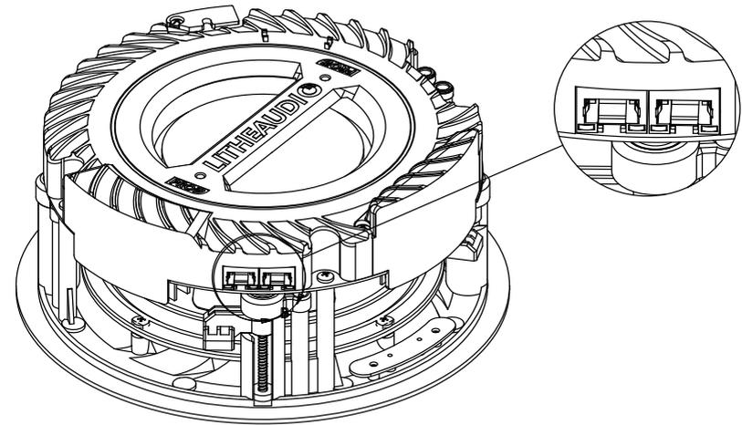
**NOTE: IF USING POE IN ADDITION TO ETHERNET CONNECTION THEY ARE SEPERATE**
