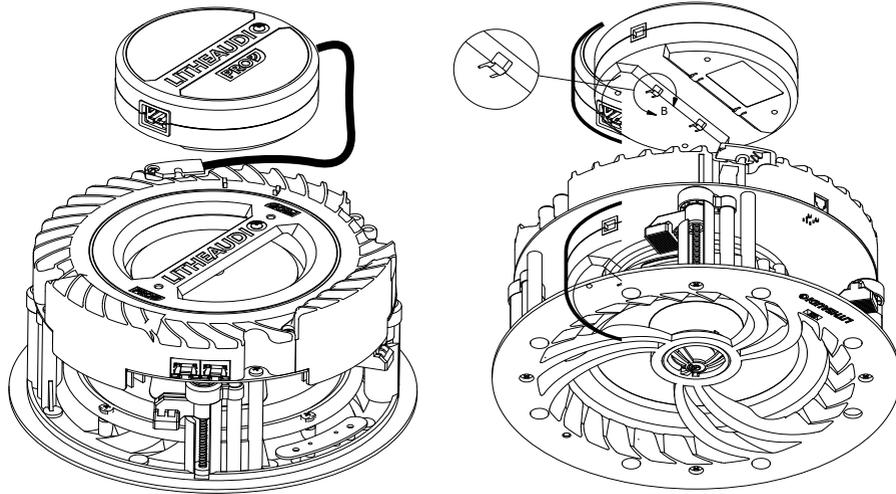
3. Connect the DC cable connector from the PoE bolt on into the speaker.
